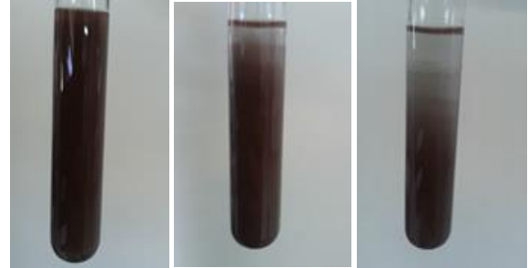
Fig. 2. 0.05 wt. % nanofluid B a) just after sonication, b) after 24 h and, c) after 4 days.
