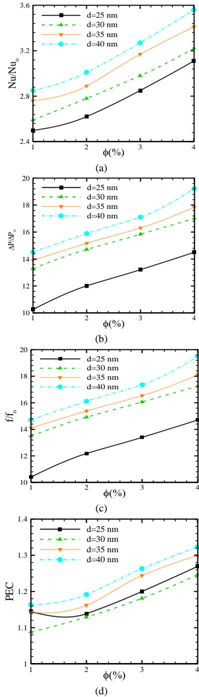
**Fig. 4** Effects of different nanoparticles diameters on thermal-hydraulic performances of studied UTC
