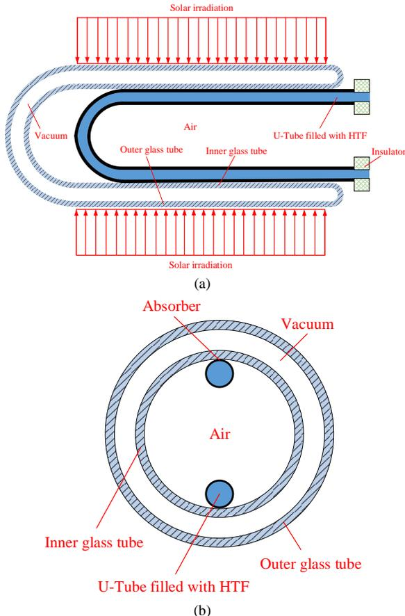
Fig.1. Schematic diagram of U-Tube solar collector: a) Front view b) Side view
