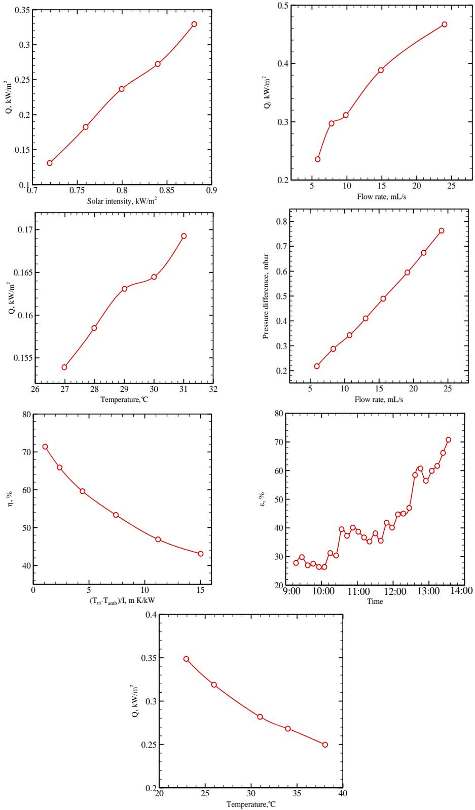
Fig. 3. Effects of using nanofluid on different parameters of studied UTC
