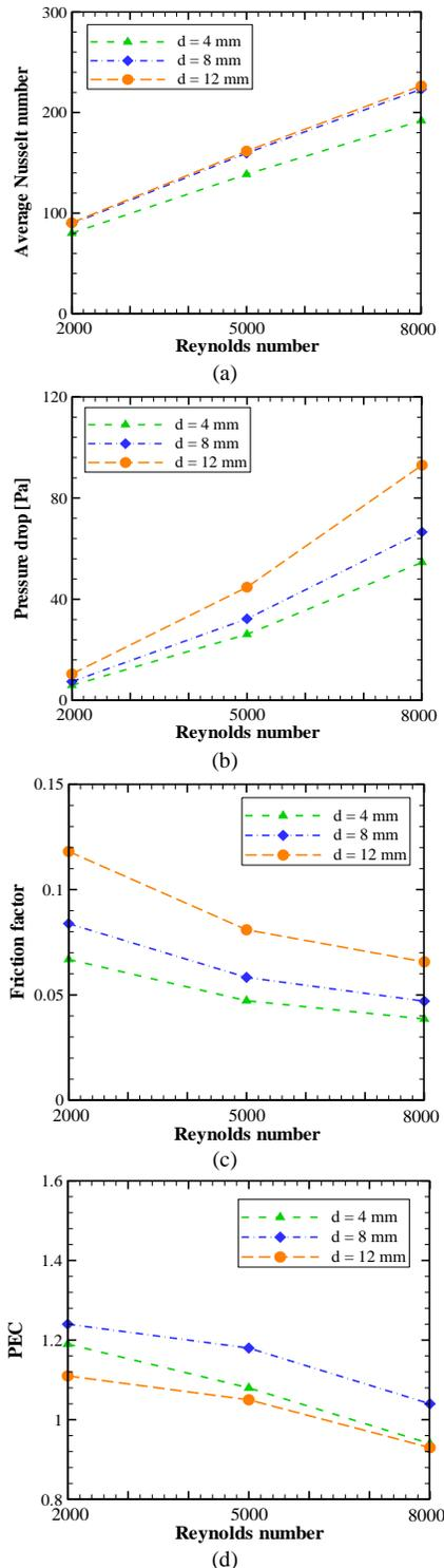
Fig. 5. Effects of different tube diameters on thermal-hydraulic performances of studied UTC
