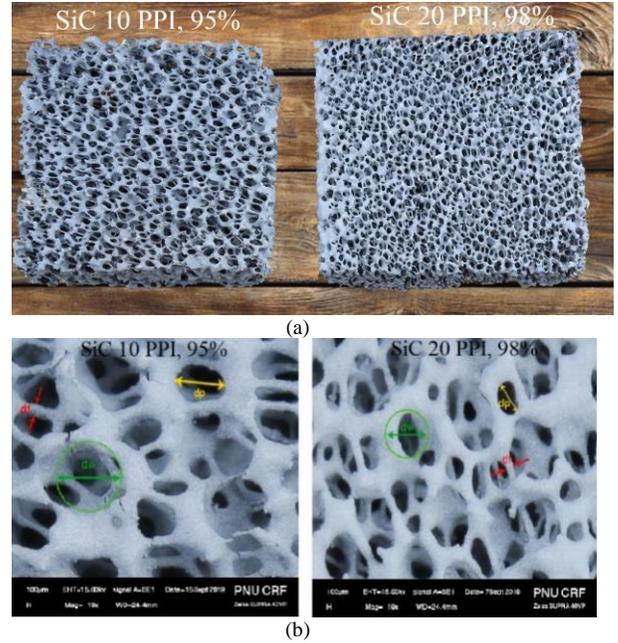
Fig. 2. (a) samples of the SiC porous foams (b) SEM images.
