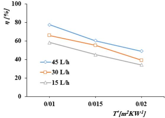
Fig. 6. Effect of the volumetric flow rate of the nanofluid on the energy efficiency. (10 PPI porous foam, the NPs concentration=500 ppm).
