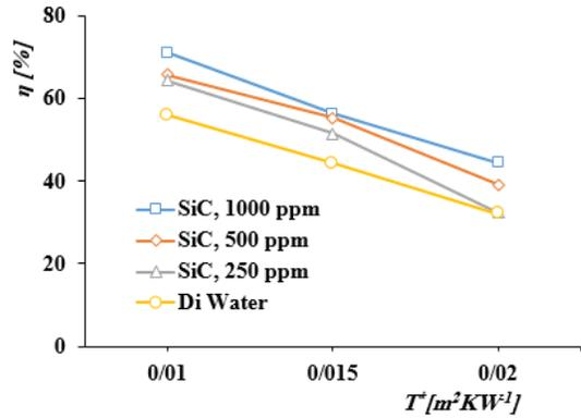
Fig. 7. Effect of the NPs concentration in the working fluid on the energy efficiency. (10 PPI porous foams, the volumetric flow rate=30  $Lh^{-1}$ )
