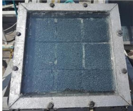
Fig. 3. Installation of the SiC foams inside the DASC.
