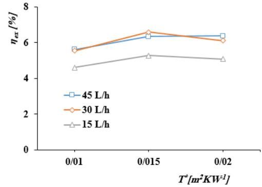
Fig. 9. Effect of the volumetric flow rate of the nanofluid on the exergy efficiency (10 PPI porous foam, the NPs concentration=500 ppm).
