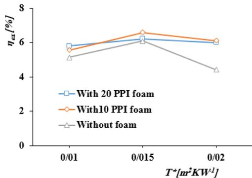
Fig. 11. Effect of installation of the porous foam and its pore density on the exergy efficiency. (The NPs concentration=500 ppm, the volumetric flow rate=30 Lh<sup>-1</sup>)
