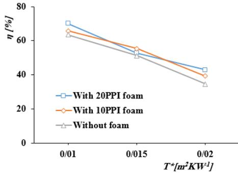
Fig. 8. Effect of installation of the porous foam and its pore density on the energy efficiency (the NPs concentration=500 ppm, the volumetric flow rate=30 Lh<sup>-1</sup>).
