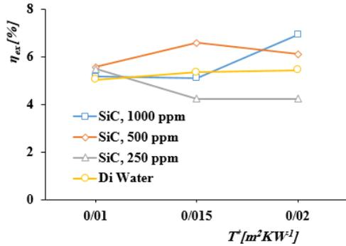
Fig. 10. Effect of the NPs concentration in the working fluid on the exergy efficiency (10 PPI porous foam, the volumetric flow rate=30 Lh<sup>-1</sup>)
