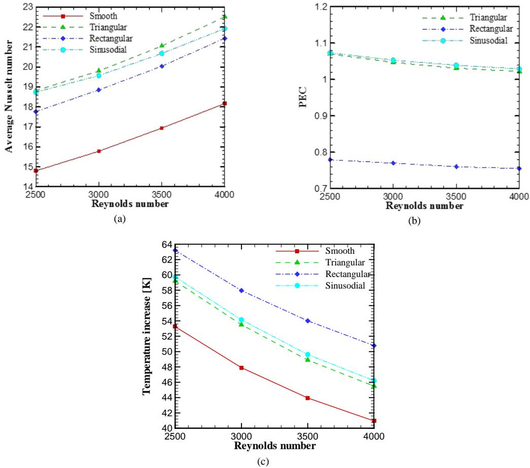
Fig. 4. Variation diagram of (a) average Nusselt number, (b) PEC, (c) air temperature increment from collector inlet to outlet, according to different Reynolds number for corrugated and smooth absorber plates during the first six months
