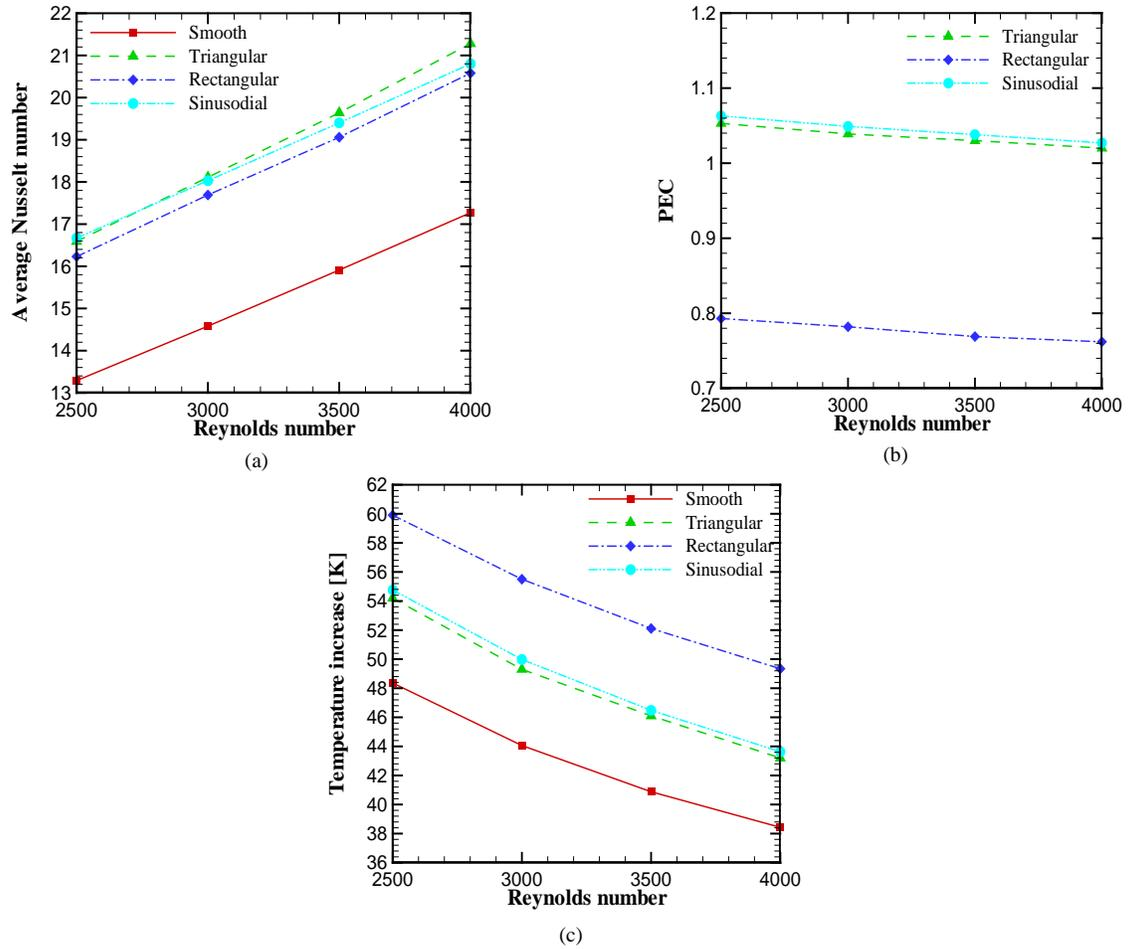
Fig. 5. Variation diagram of (a) average Nusselt number, (b) PEC, (c) air temperature increment from collector inlet to outlet, according to different Reynolds number for corrugated and smooth absorber plates during the second six months
