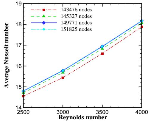
Fig. 2. Average Nusselt number variation diagram according to Reynolds number for different grid sizes in smooth absorber plate
