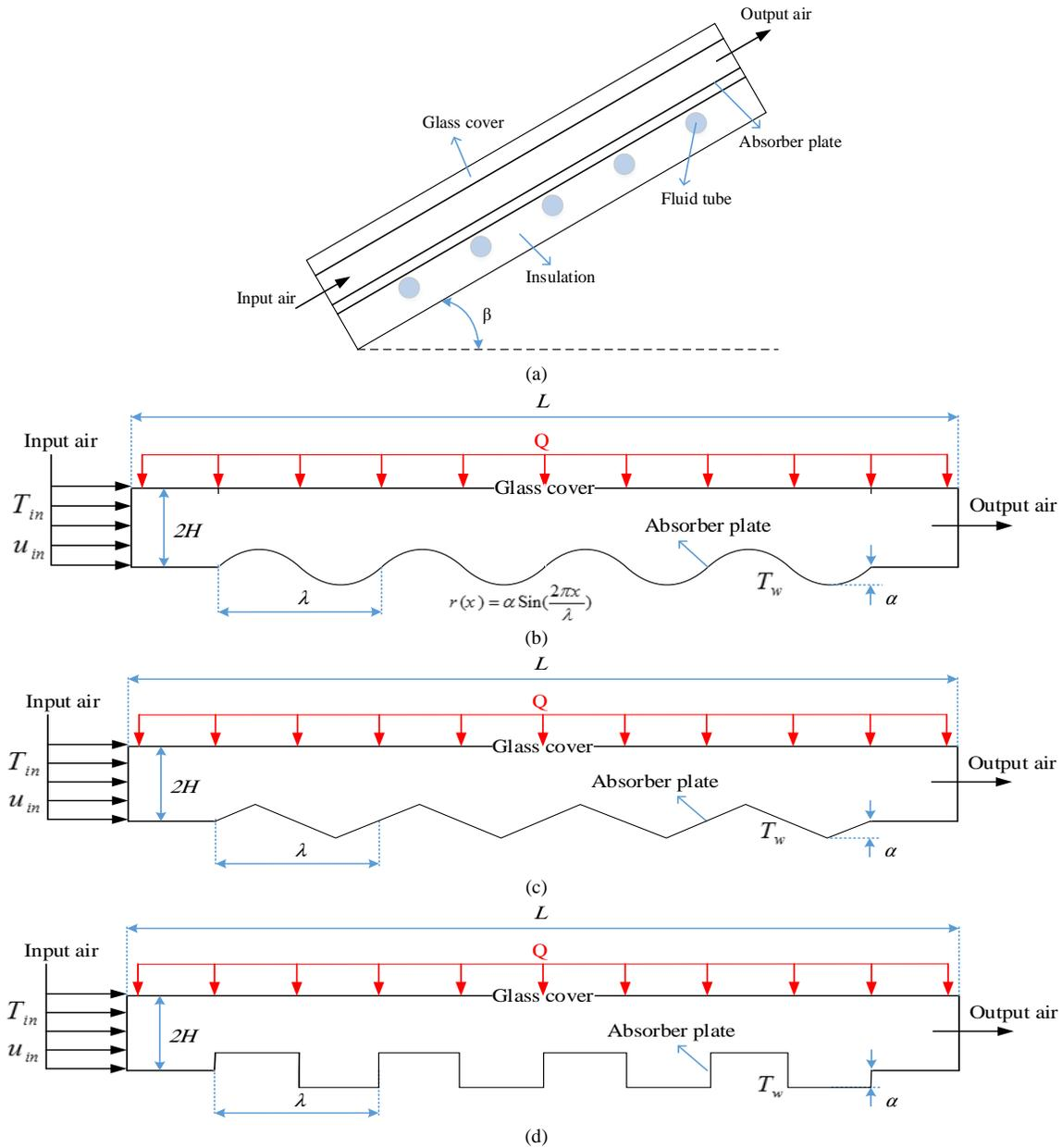
**Fig. 1.** (a) The schematic diagram of the two dimensional collector with double application. Two dimensional solar collector models with: (b) sinusoidal corrugation, (c) triangular corrugation, and (d) rectangular corrugation. (The actual geometry consists of 18 corrugations but for clear presentation only 4 waves have been shown.)
