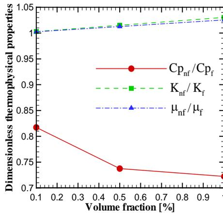
Fig. 6. Non-dimensional specific heat, thermal conductivity and dynamic viscosity according to carbon black nanoparticle volume fraction in nanofluid mixture
