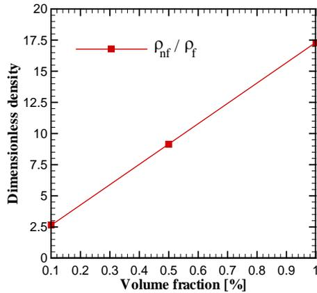
Fig. 7. Non-dimensional density variation according to carbon black nanoparticle volume fraction in nanofluid mixture
