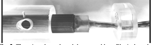
Fig. 2. The microchannel module covered by a Plexi-glass shell
