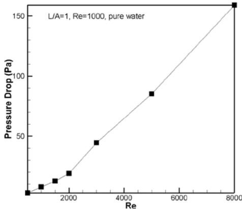
Fig. 7. The effect of Reynolds number on channel pressure drop
