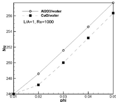
Fig. 12. The effect of nanoparticle's type on average Nusselt number
