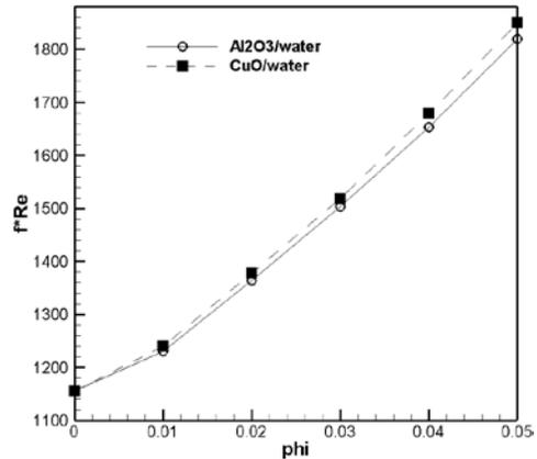
Fig. 13. The effect of nanoparticle's type on pressure drop
