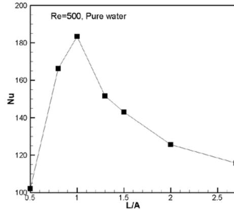
Fig. 5. The effect of plate sine wave pattern on average Nusselt number
