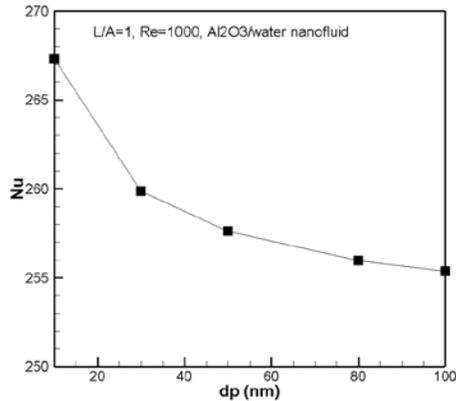
Fig. 11. The effect of nanoparticle's diameter on average Nusselt number
