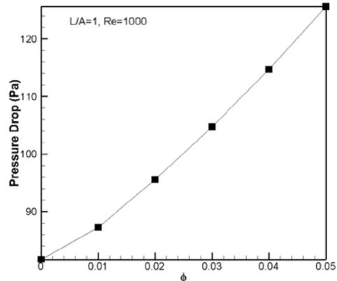
Fig. 10. The effect of volume fraction of nanoparticles on channel pressure drop
