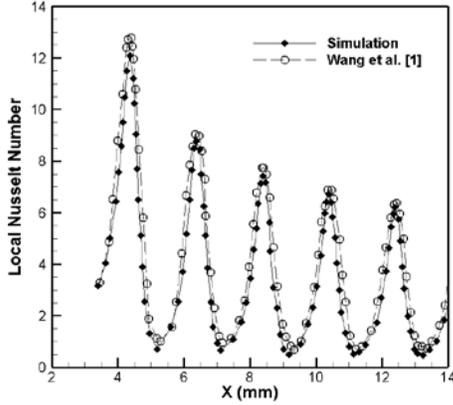
Fig. 2. Verification study for local Nusselt number for a wave channel in the laminar fluid flow
