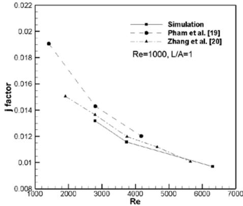
Fig. 3. Verification study for the Colburn factor j for a wave channel in turbulent fluid flow
