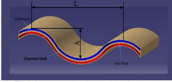
Fig. 1. Geometry and boundary condition of the problem
