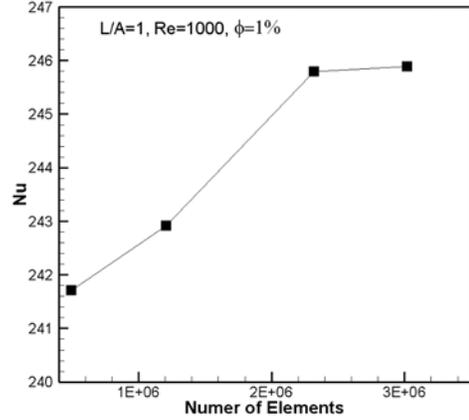
Fig. 4. Average Nusselt based on the number of computational cells
