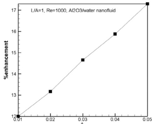
Fig. 9. The effect of volume fraction of nanoparticles on Nusselt number enhancement
