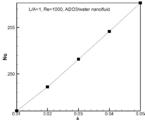
Fig. 8. The effect of volume fraction of nanoparticles on average Nusselt number
