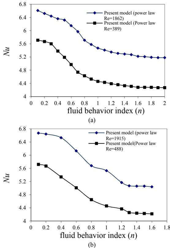
**Fig. 4.** (a) Simulation  $Nu$  number as function of  $n$  for 2 Vol %  $Al_2O_3$  nanofluid (for  $Re=1862$ ,  $Nu_{exp}=5.050$  and for  $Re=389$ ,  $Nu_{exp}=4.104$ ) (b) Simulation  $Nu$  number as function of  $n$  for 0.5 Vol %  $Al_2O_3$  nanofluid (for  $Re=1915$ ,  $Nu_{exp}=4.858$  and for  $Re=488$ ,  $Nu_{exp}=3.961$ )
