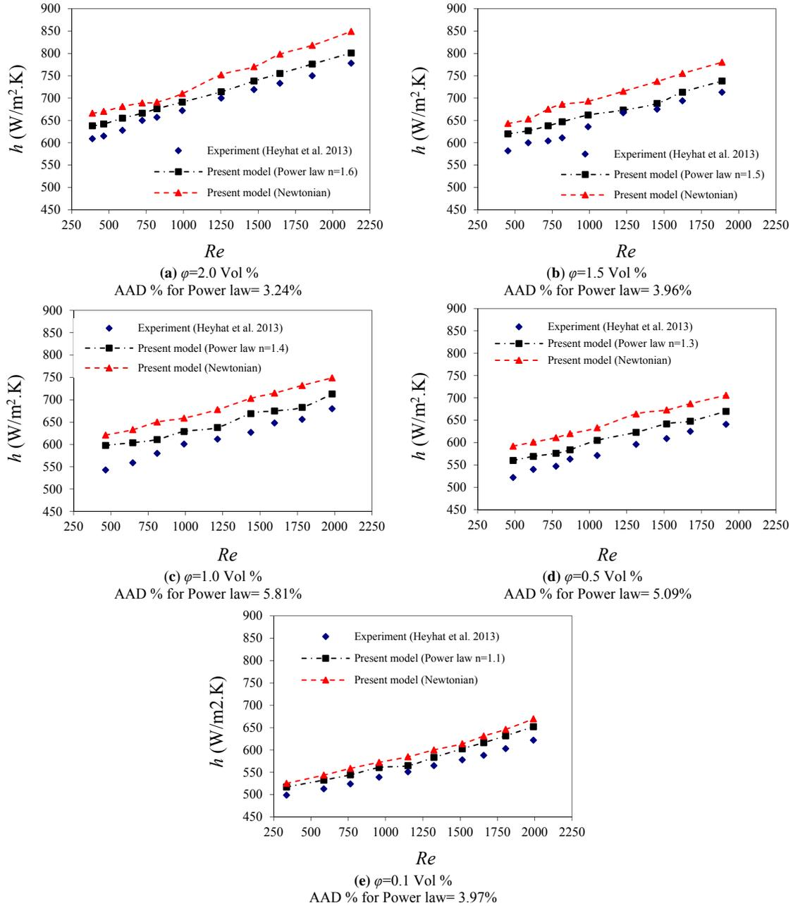
**Fig. 5.** Comparison of experimental average heat transfer coefficient [15] and the simulated results by power-law and the Newtonian model (a)  $\phi=2.0$  Vol % (b)  $\phi=1.5$  Vol % (c)  $\phi=1.0$  Vol % (d)  $\phi=0.5$  Vol % (e)  $\phi=0.1$  Vol %
