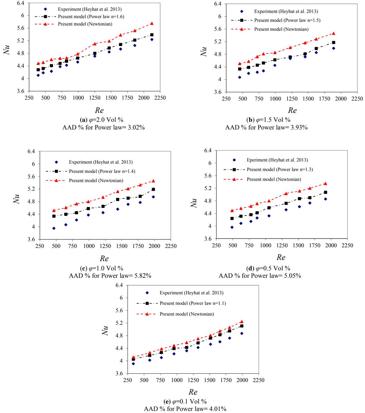
**Fig. 6.** Comparison of experimental average Nusselt number [15] and the simulated results by power-law and the Newtonian model (a)  $\phi=2.0$  Vol % (b)  $\phi=1.5$  Vol % (c)  $\phi=1.0$  Vol % (d)  $\phi=0.5$  Vol % (e)  $\phi=0.1$  Vol %
