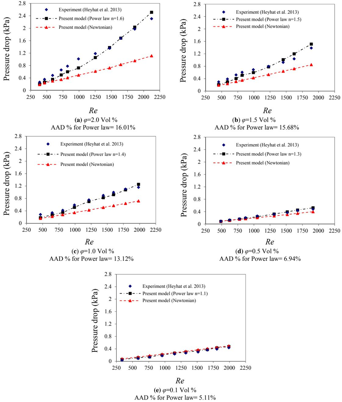
Fig. 7. Comparison of experimental pressure drop [15] and the numerical simulation results by power-law and the Newtonian model (a)  $\phi=2.0$  Vol % (b)  $\phi=1.5$  Vol % (c)  $\phi=1.0$  Vol % (d)  $\phi=0.5$  Vol % (e)  $\phi=0.1$  Vol %
