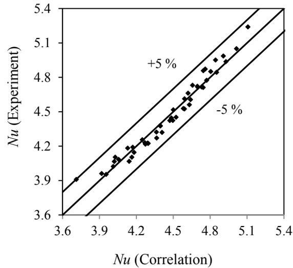
Fig. 8. Comparison of experimental [15] and correlation (Eq. 14) Nusselt number for  $Al_2O_3$  nanofluid
