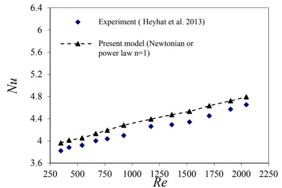
Fig. 2. Experimental [15] and the simulation data for average Nusselt number of pure water
