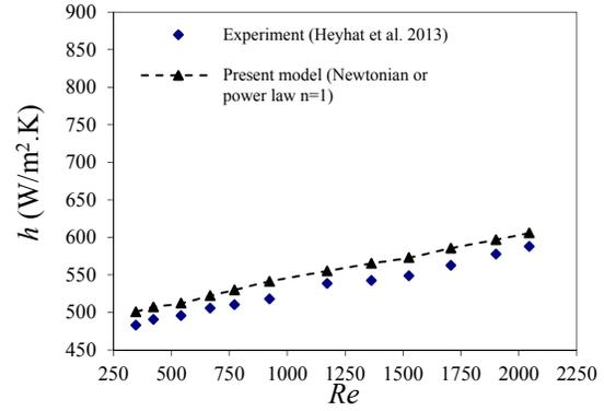
Fig. 1. Experimental [15] and the simulation data for heat transfer coefficient of pure water
