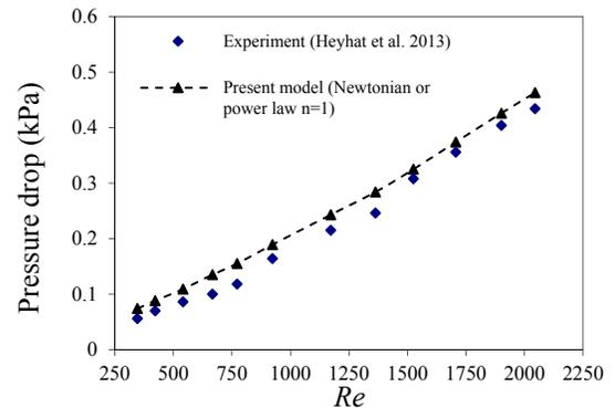
Fig. 3. Experimental [15] and the simulation data for pressure drop of pure water
