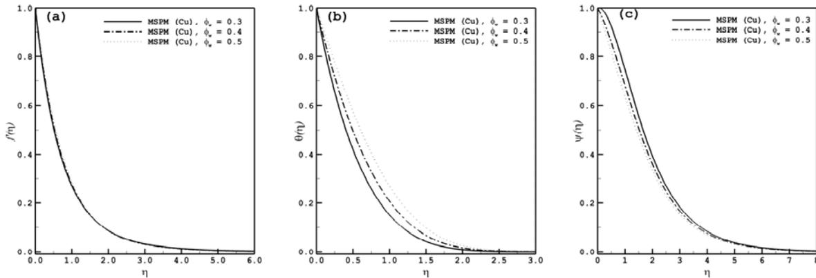
Fig.6. Effect of  $\varphi_w$  on the dimensionless profiles ( $f, \theta, \psi$ ) for Cu-water nanofluids,  $n = 5$ , and  $r = 5$ .
