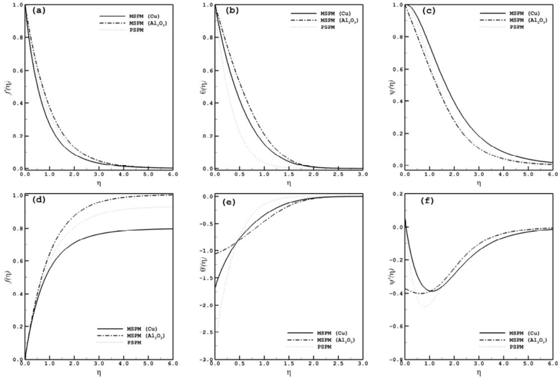
**Fig. 3.** Effect of the MSPM and PSPM on the dimensionless profiles ( $f, f', \theta, \theta', \psi, \psi'$ ) for Cu and Al<sub>2</sub>O<sub>3</sub>-water nanofluids,  $n = 5$ , and  $r = 5$
