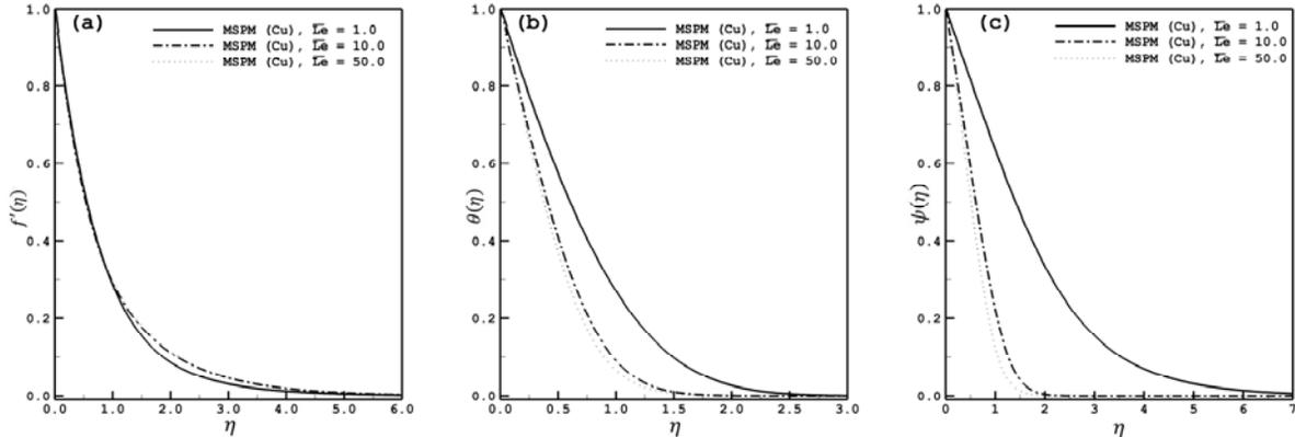
Fig. 5. Effect of  $\overline{Le}$  on the dimensionless profiles ( $f, \theta, \psi$ ) for Cu-water nanofluids,  $n = 5$ , and  $r = 5$
