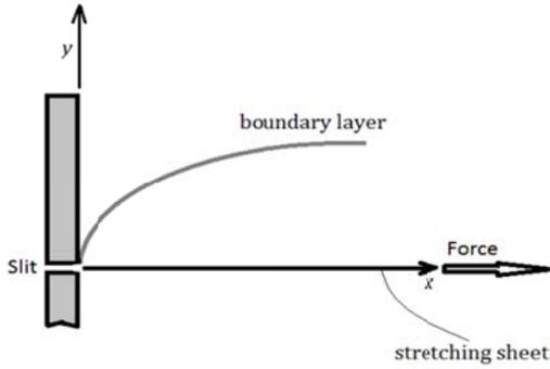
Fig. 1. Physical model of BLF of a nanofluid past a stretching sheet and coordinate system
