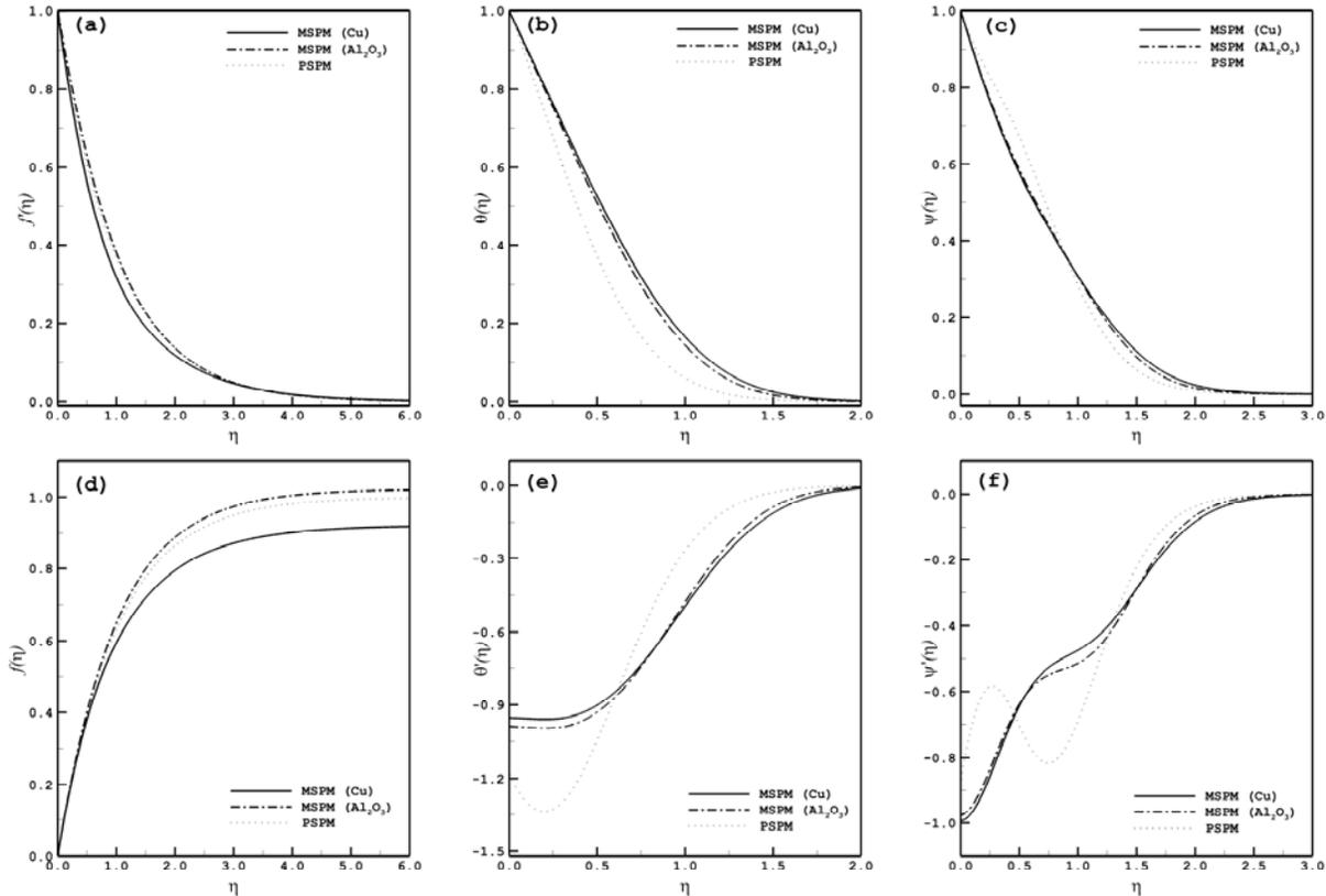
Fig. 2. Effect of the MSPM and PSPM on the dimensionless profiles ( $f, f', \theta, \theta', \psi, \psi'$ ) for Cu and  $Al_2O_3$ -water nanofluids,  $n = 1$ , and  $r = 0$
