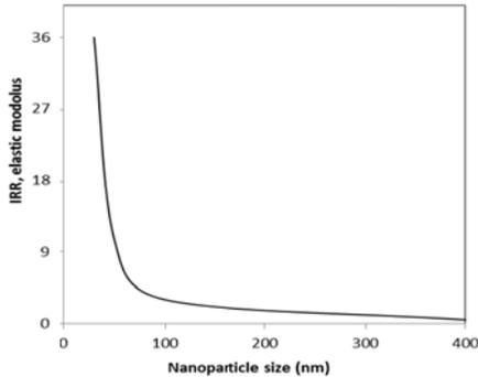
Fig. 13.  $IRR$  for elastic modulus of nanocomposite for different size of nanofiller. Interphase thickness is considered to be 30 nm
