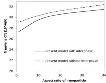
Fig. 11. Variation of transverse CTE with change in aspect ratio of silica nanofiller
