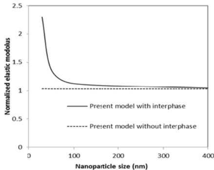
Fig. 5. Effect of nanoparticle size on the elastic modulus of nanocomposite
