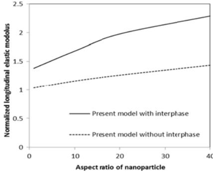
Fig. 8. Variation of longitudinal elastic modulus with change in aspect ratio of silica nanofiller
