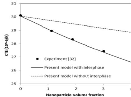
**Fig. 4.** Variation of CTE with change in volume fraction of silica nanoparticle
