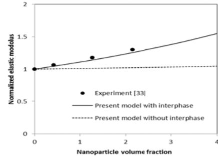
**Fig. 3.** Variation of elastic modulus with change in volume fraction of silica nanoparticle
