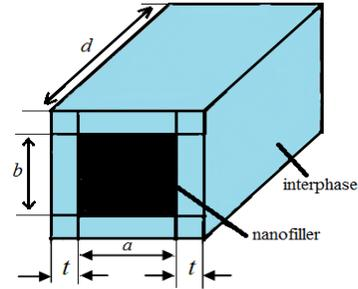
Fig. 2. Cell including nanoparticle
