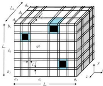
Fig. 1. RVE in the modified SUC model for nanocomposite materials
