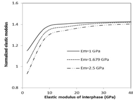
Fig. 15. Effects of polymer matrix properties on the elastic modulus of nanocomposite
