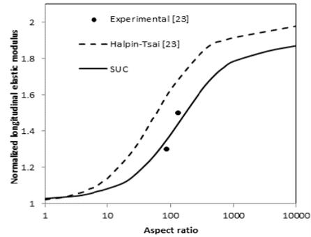
Fig. 7. Variation of longitudinal elastic modulus of nylon-6/clay nanocomposites with change in clay aspect ratio
