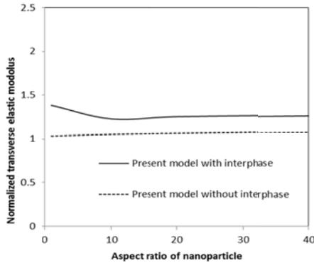
Fig. 9. Variation of transverse elastic modulus with change in aspect ratio of silica nanofiller
