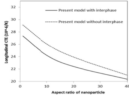
Fig. 10. Variation of longitudinal CTE with change in aspect ratio of silica nanofiller
