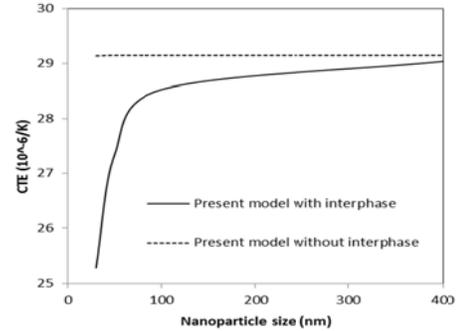
Fig. 6. Effect of nanoparticle size on CTE of nanocomposite
